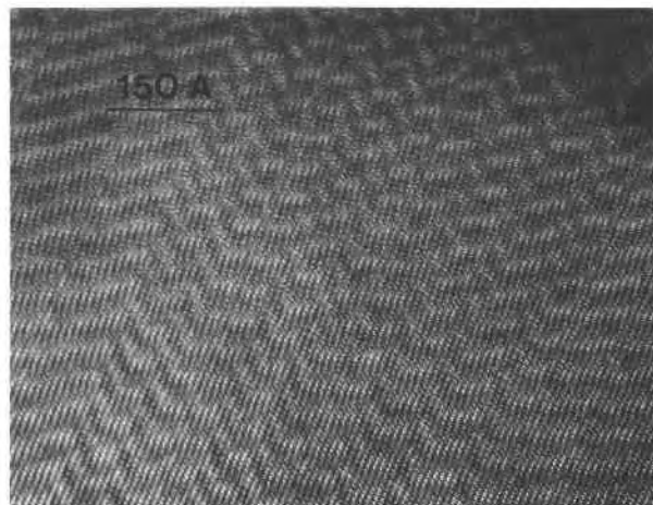
Fig. 9. Lattice image of sartorite down [010] showing domains of ordered twinning of the structural modulation, which range from 50 up to 150 Å in width.
