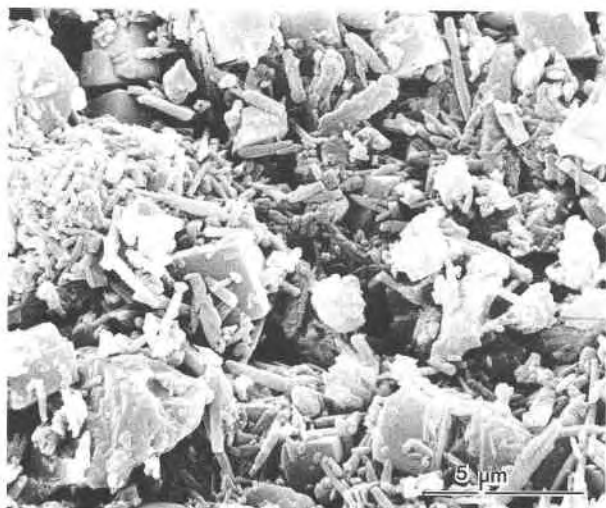
Fig. 1. SEM image of an intertidal carbonate assemblage from the Abu Dhabi sabkha (AD 31). Shown are aragonite needles and dolomite and magnesian calcite rhombs.
