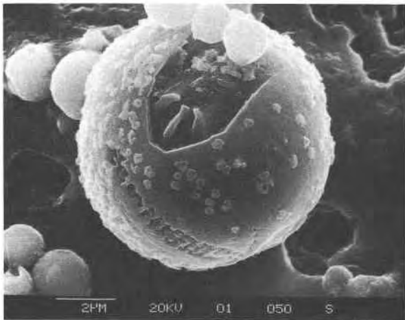
Fig. 2. Secondary electron image of a microsphere showing typical prismatic structure in the outer layer, with angular outline and three radial features. Representative compositions for the inner and outer shells are given in Table 1. Note band with graphic texture along lower left side of sphere.
