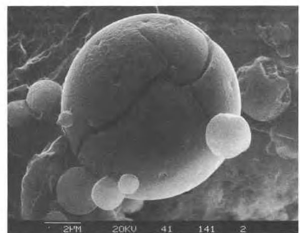
Fig. 5. Secondary electron image of high-silica microsphere with cracked shell and regularly spaced oxides on surface.
