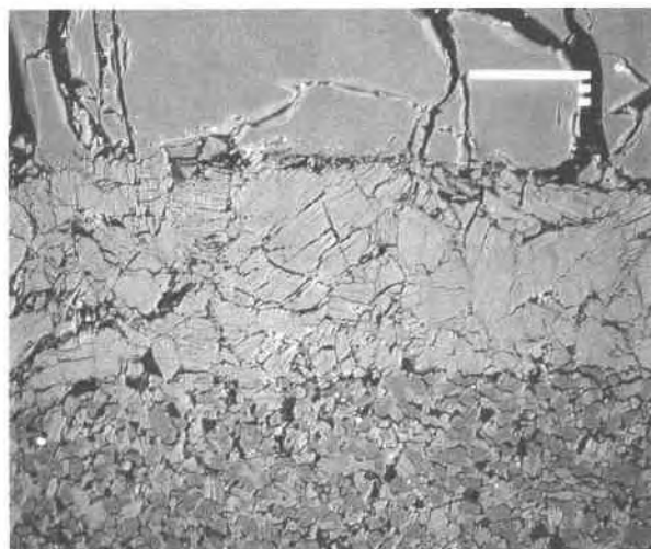
Fig. 2. Backscattered electron image of an experimental product from melting experiments with carbonate flux (expt. 1898, 13 GPa, 1950 °C). Shown in the sequence with decreasing temperature from the top is the melt, preserved as brown transparent glass, a layer of Ca 2 SiO 4 , produced by incongruent melting and segregated from the melt, and the subsolidus assemblage of Ca 2 SiO 4 + CaSi 2 O 7 at the bottom. The scale is 100 μm long.
