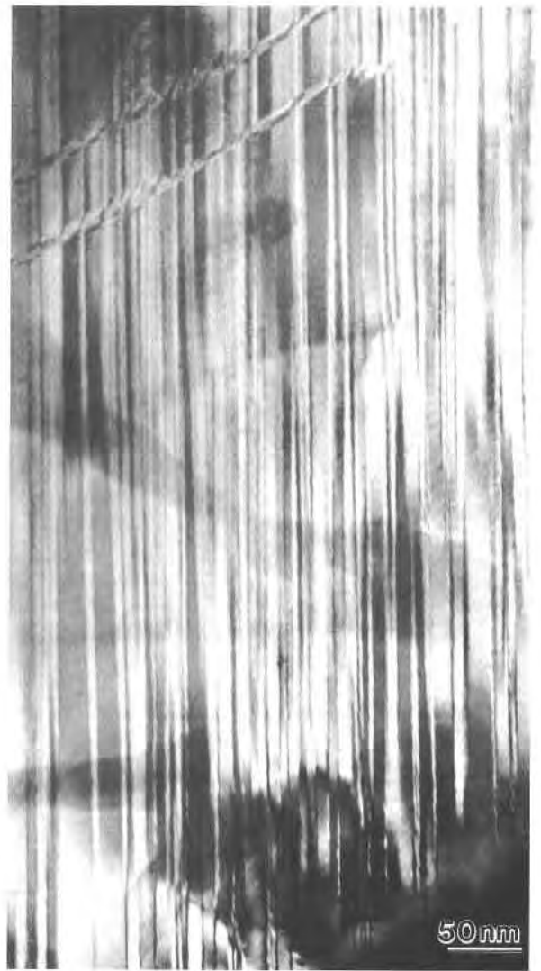
Fig. 14. Dark-field image formed using the 242 reflection for an area showing a well-developed maghemite superstructure (diffraction pattern shown in Fig. 6b). Alternating regions with dark and light contrast separated by defects may be due either to strain contrast or to maghemite in twin-related orientations.
