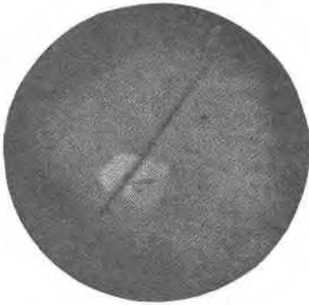
FIG. 5. Passed thru 200-mesh screen. White, pentlandite; gray, pyrrhotite; black, wax. Magnification 580 \times .
