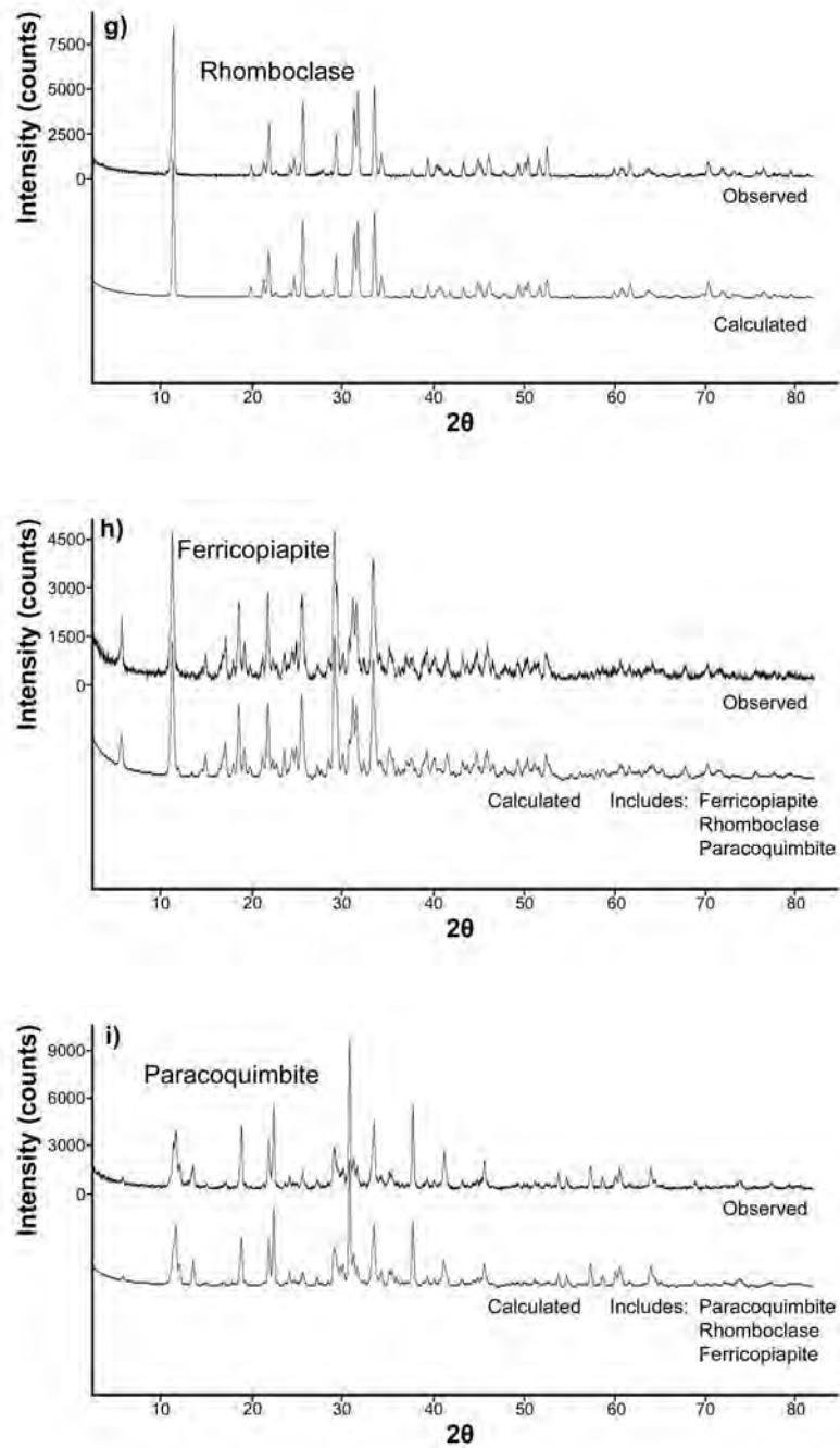
Deposit<sup>2</sup>. a)-i). XRD patterns a-f with matching patterns from the ICDD database. XRD patterns g-i with calculated patterns from known crystal structures. a) szomolnokite, b) melanterite, c) schwertmannite, d) jarosite, e) hematite, f) magnetite, g) rhomboclase, h) ferricopiapite, i) paracoquimbite.
