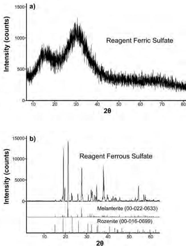
Deposit<sup>1</sup>. XRD patterns of reagents with matching patterns from the ICDD database. a) reagent ferric sulfate, b) reagent ferrous sulfate.
