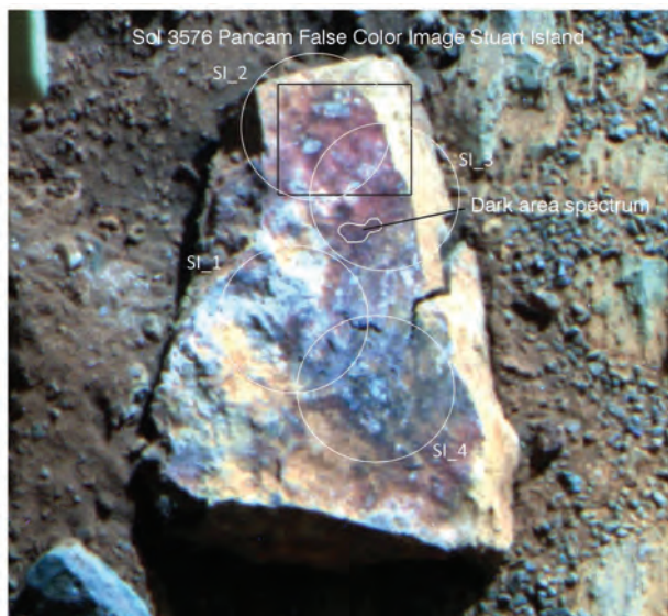
FIGURE 16. Pancam false color image of Stuart Island acquired on sol 3567 showing the locations and 100% field of view of the four APXS observations. Box delineates location for the MI-based anaglyph shown in Figure 17. The location is denoted from which a dark area spectrum derived from Pancam data is shown in Figure 18. For reference Stuart Island is about 0.12 m in its long dimension. Pancam product IDs 1P445650967RADCAGYP2539L2C1, 1P445651052RADCAGYP2539L5C1, and 1P445651127RADCAGYP2539L7C1.
