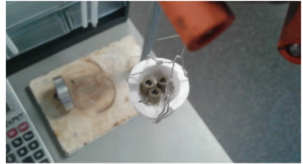
FIGURE 4. Three Fo.70 capsules hosting martian (iron-rich) basaltic melts, as they appear shortly after their removal from the furnace. Reflections from the concave melt pools are clearly visible. The capsules shown here are supported by an alumina crucible, with a platinum grill holding them above the crucible base (so that they do not fuse themselves to it), but it is also, of course, possible to suspend the capsules in individual platinum cages.
