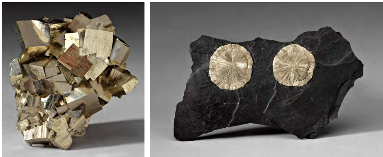
FIGURE 1. (left) Coarse grained pyrite showing the distinctive cubic form. (right) Pyrite nodule in shale. Both photos provided by the Royal Ontario Museum.
