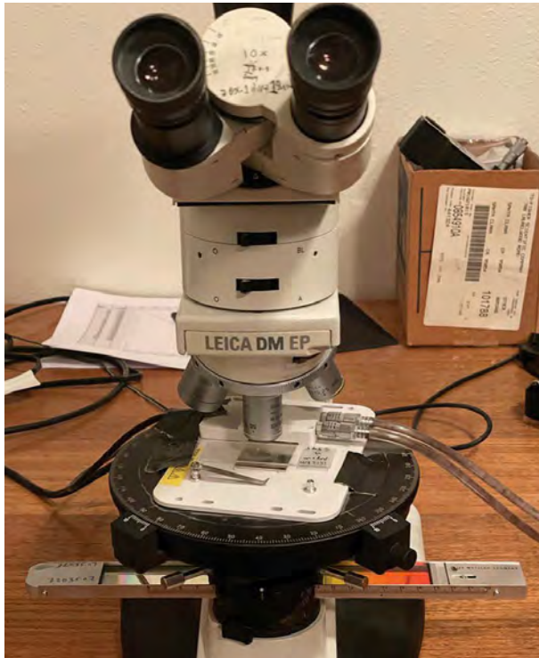
FIGURE 3. A polarizing light microscope equipped with a heating/cooling stage and monochromator. This is the setup used herein to employ the double variation method for precise refractive index determination.
