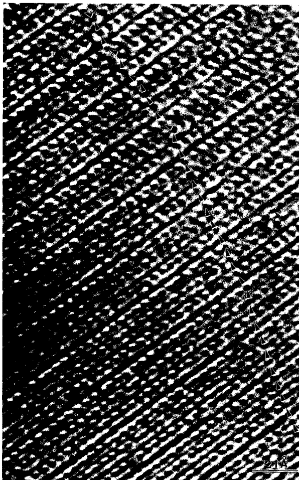
Fig. 6. HRTEM image down [100] of a typical well-ordered crystal. Note the abundant b/3 displacement disorder within 2:1 layers, between 2:1 and serpentine layers, and across the brucitic interlayer (illustrated by the random displacements of the dark spots).
