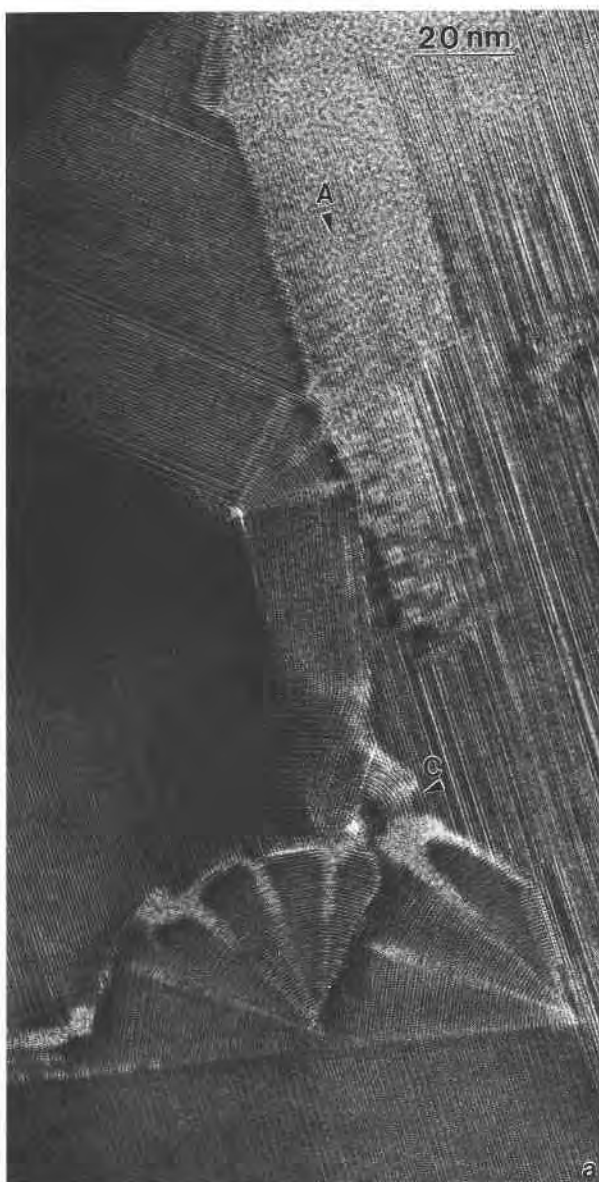
Fig. 14 (above and right). The [100] images of polygonal serpentine. (a) Polygonal segments bridge planar serpentine. Beam damage is concentrated at segment interfaces. A indicates antigorite, and C indicates chrysotile-like serpentine. (b) Polygonal serpentine developed at grain boundaries between planar serpentine-chlorite intergrowths. Arrows in the top right corner indicate that (inclined) planar faults on (100) may be antiphase boundaries between chlorite units and separate serpentine and chlorite.
