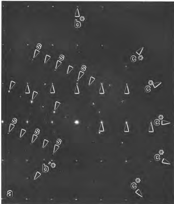
Fig. 16. Diagram illustrating the polytypic structure of polygonized serpentine as inferred from SAED patterns.
