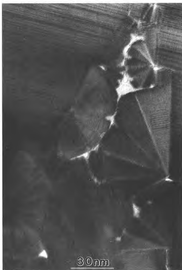
Fig. 13. Image down [100] illustrating polygonal serpentine in a zone that crosscuts planar serpentine. Polygonal crystals appear to have nucleated at steps on the surface of the planar serpentine.
