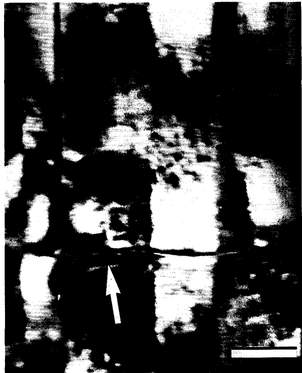
Fig. 4. Same sample as in Fig. 2. Tweed texture. Large albite twins demonstrate the triclinic symmetry of the grain; a pericline lamella is shown by the arrow. Dark field, g = 062 ; scale bar: 0.1 \mu\text{m} .
