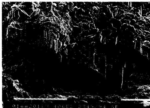
FIGURE 1. SEM photo of fianelite crystals. Notice the strong striation parallel to the a axis. Field of view is \sim 0.25 mm.
