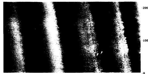
FIGURE 10. Two STM images of a fresh pyrite fracture surface, tiled together. White arrows indicate two images of the same step edge, the result of a double-tip artifact that manifests itself on all the steps. Total vertical relief in these images is 1.5 nm, and the steps are (after accounting for artifacts) about 1 nm high, or two unit cells. Numbered scales in nanometers. Conditions: 1.0 nA, 400.0 mV.
