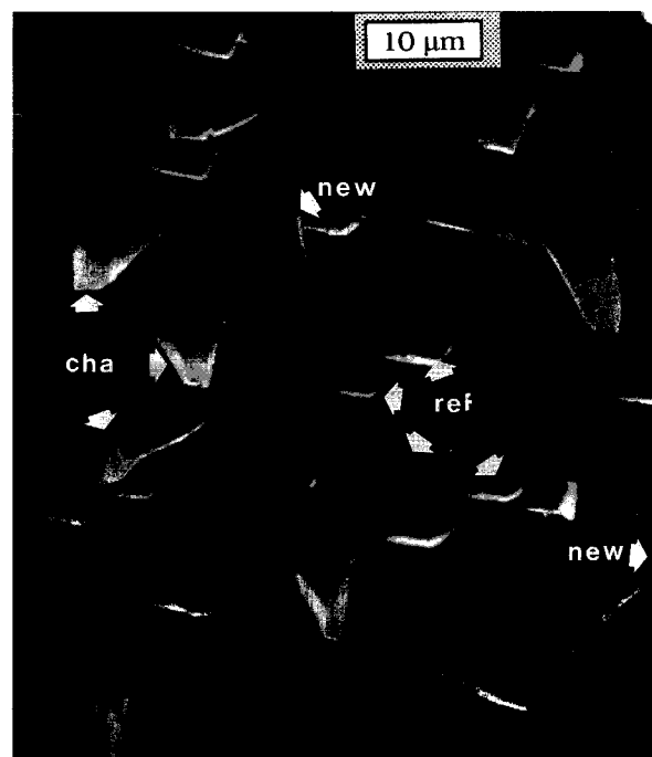
FIGURE 16. The track channels (cha) in \{11\bar{2}0\} (S type) are nearly wedge shaped at a low etchant concentration (0.25% \text{HNO}_3 ). The needle-shaped channels (new) correspond to tracks that were added as a result of bulk etching. Residual etch figures (ref) are clearly developed at this concentration. Etching conditions: 1800 s in 0.25% \text{HNO}_3 (set D).
