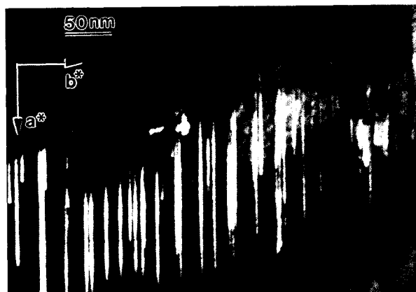
FIGURE 3. A dark-field image of tremolite quenched from 740 °C produced by selecting a streaked diffraction maxima at 110^* , showing (010) clinopyroxene slabs.
