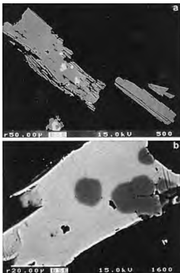
FIGURE 1. Backscattered electron images of synthesis and reversal experiment products: (a) synthetic Opx with 5 wt% \text{Al}_2\text{O}_3 ; bright spots are fayalite nuclei; (b) almandine (dark spots) and Opx (bright matrix) intergrowth in experiment 2b.
