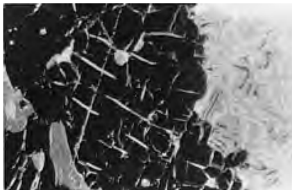
FIGURE 3. Cathodoluminescence photomicrograph showing plagioclase (grey) and wollastonite (white) symplectite after scapolite, and garnet (black) cut by wollastonite filled fractures (width of view ~0.7 mm).
