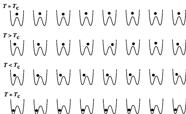
FIGURE 6. Sequence showing the ordering of atoms for the model of Figure 3 in the displacive limit. At high temperatures ( T \gg T_c , \eta = 0 ) the atoms vibrate about the zero position, and the effects of the double-well potential are not significant. On cooling toward the transition temperature ( T > T_c , \eta = 0 ) the effects of double-well potential become more significant and a degree of short-range order is established, where neighboring groups of atoms are temporarily slightly displaced from the origin. Below the transition temperature ( T < T_c , |\eta| > 0 ) the atoms vibrate about positions that are shifted away from the origin, and all atoms vibrate about the same displaced point. At very low temperatures ( T \ll T_c , \eta = \eta_0 ) all the atoms occupy the same side of the double-well potential.
