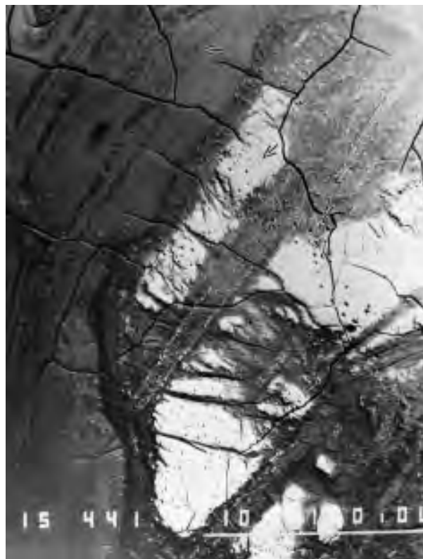
FIGURE 3. Backscattered electron image of relict uraninite (bright contrast) partly replaced by clarkeite and K-rich phase (darkest contrast). Bubbles in the uraninite are preserved in the surrounding clarkeite (arrows), suggesting solid-state replacement (sample DMNH 13283). Scale bar at lower right is 100 μm.
