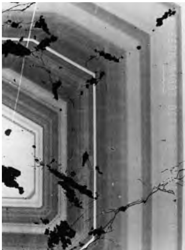
FIGURE 5. Backscattered electron (BSE) image of garnet crystal K92-2. The andradite-rich sections are light, whereas the grossular-rich sections are dark. The horizontal scale is 9 mm.
