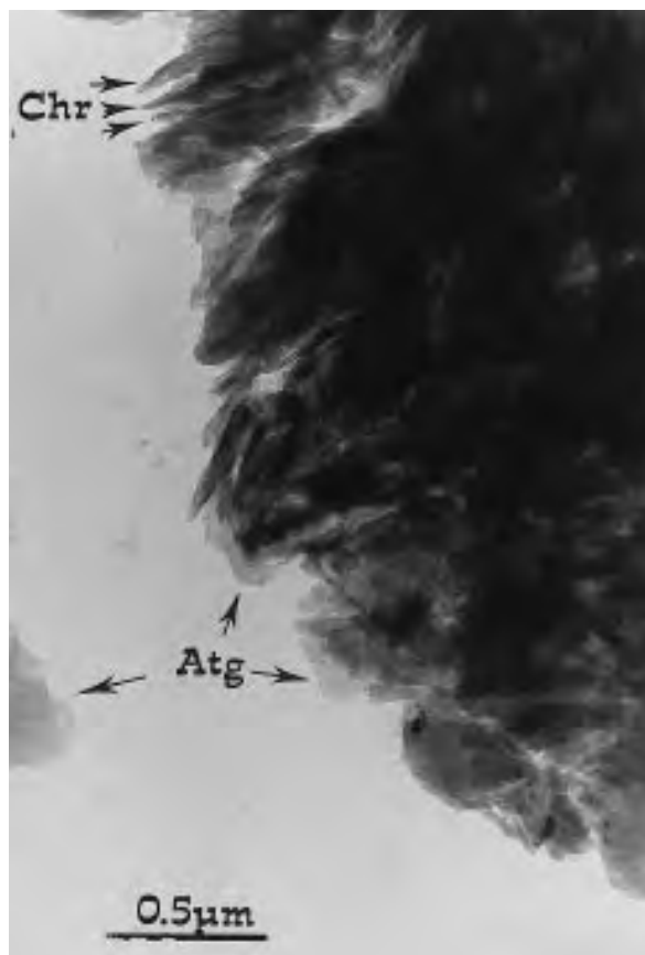
FIGURE 3. Low-magnification TEM image of the products of experiment 254. Chr = chrysotile rolls with hollow cores; Atg = antigorite crystals.
