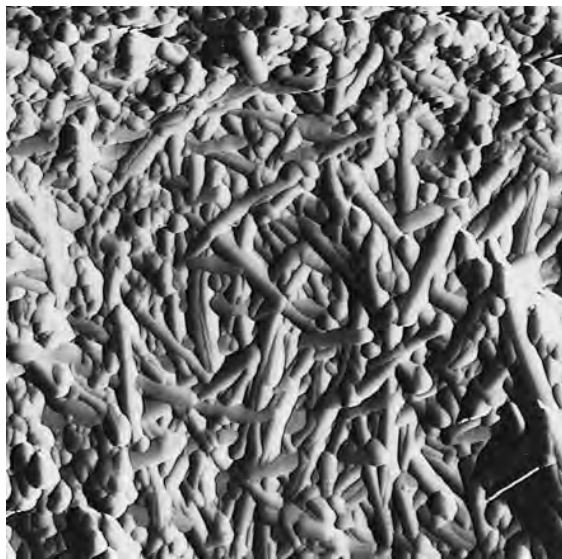
FIGURE 6. HAP reacted with 500 mg/L [Pb_{aq}]_i . TMAFM image showing botryoidal masses (see top portion of image) and small intergrown needles (scan area = 2.00 \mu\text{m} on a side). SEM (results not shown) revealed aggregates of morphologically indistinct material. XRD results (see Fig. 3e) indicate that the sample was HPY. EDS (results not shown) indicate that the material imaged with SEM was dominated by Pb and P.
