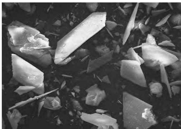
FIGURE 2. SEM of hydroxylapatite (HAP) reactant used in batch sorption experiments showing plate-like particles of various sizes (image size = 570 × 410 μm).
