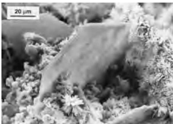
FIGURE 1. SEM photograph of a thin, tabular gordaite crystal of hexagonal habit, associated with tiny barite aggregates from the Juan de Fuca Ridge, northeastern Pacific Ocean.
