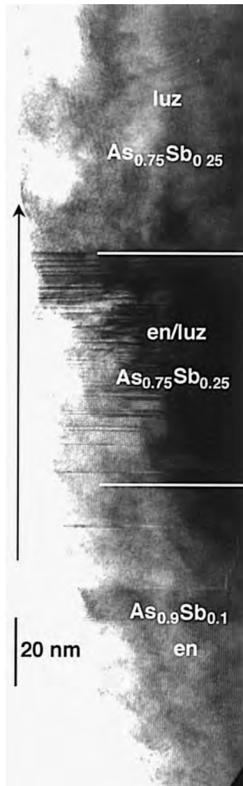
FIGURE 3. Intergrowth of enargite and luzonite. The atoms per formula unit are shown for As and Sb for both phases. A structurally disordered zone is marked "en/luz." The arrow shows the assumed direction of crystal growth (see Discussion).
