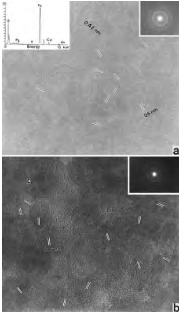
FIGURE 7. HRTEM image of goethite. (a) HRTEM image of thick-banded ore. The lattice fringes of 0.5 nm and 0.42 nm correspond to d spacings of (020) and (111) planes of goethite, respectively. (b) HRTEM image of goethite grains in thick-banded ore. Right hand part corresponds to light contrast part ( L_2 ) and left hand part is thick mineralized part ( D ).
