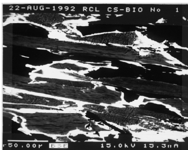
FIGURE 1. Backscattered-electron image of subparallel platy crystals of phlogopite (dark grey) with outer zones enriched in Rb and Cs (white), in plagioclase and quartz (black). The scale bar is 50 μm long.
