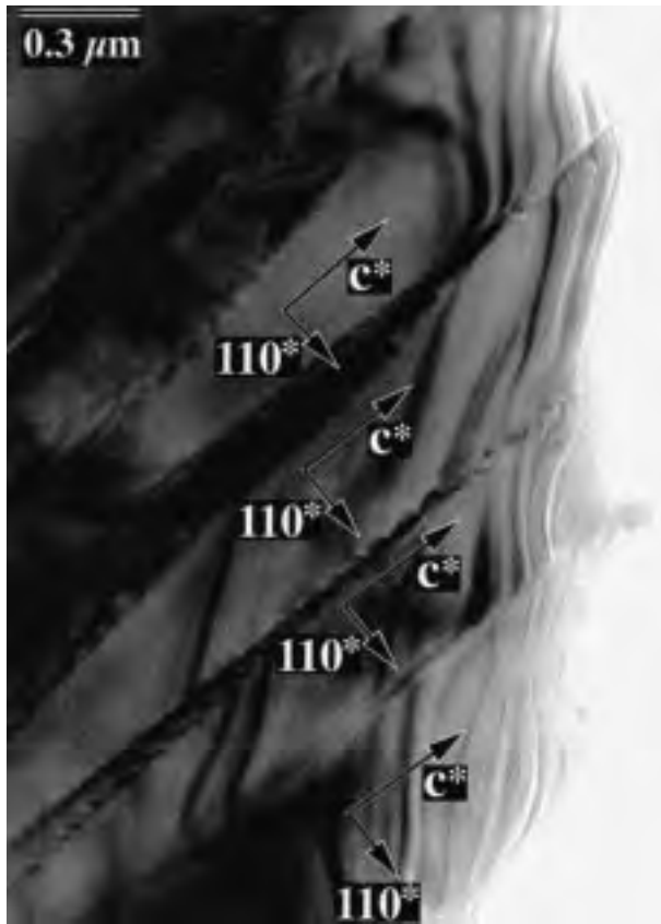
FIGURE 1. TEM micrograph showing a typical area of fibrolite from Lewiston, Idaho.
