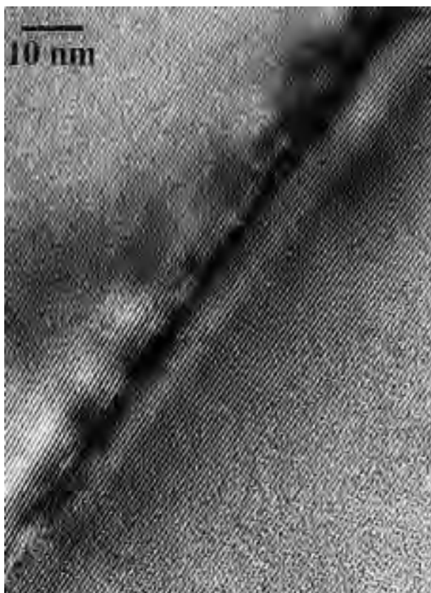
FIGURE 5. TEM micrograph of a low-angle tilt boundary between two grains of fibrolite where the angle of mismatch between the c axes of each grain is 5^\circ . Edge dislocations can clearly be seen if the image is viewed from a low angle.
