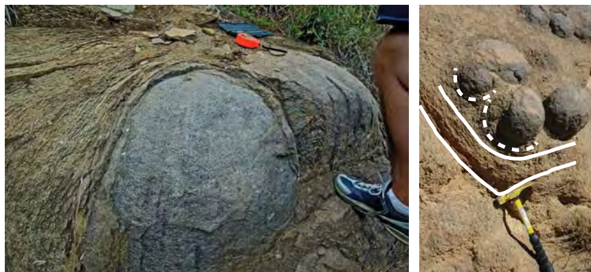
Figure 1. Spheroidal weathering of doleritic sill intrusion from the Karoo Basin, South Africa. Reaction-driven fracturing produces a number of spalls (‘onion-skin’-like fractures) that result in a rounded ‘core stone’ from an initially angular dolerite block, cut out by pre-existing joints (left). Continued weathering eventually produces tensile stresses inside the core stone that are high enough to make the original core stone (outlined by solid lines) divide into two or more daughters (dashed lines) (right). [Modified from Røyne et al. 2008].
