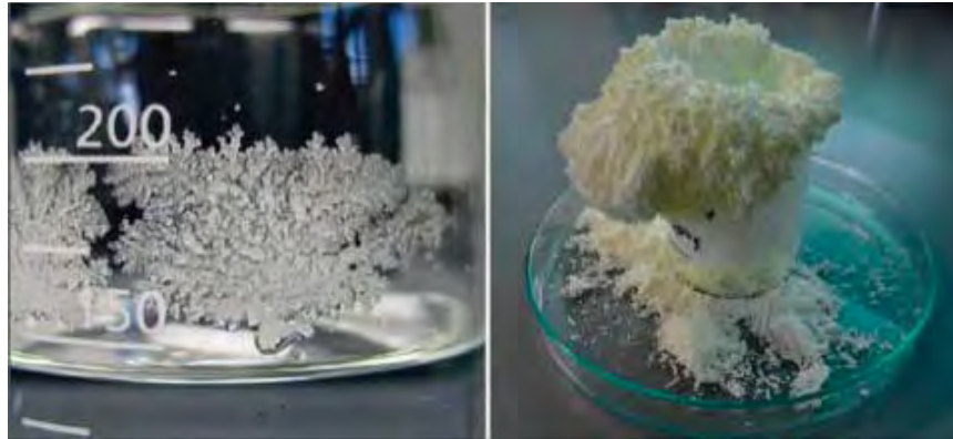
Figure 12. Creeping of a saturated NaCl solution, first as a thin layer of crystals on the side of the beaker (left) followed by secondary creeping on the first structure that formed, leading to a porous mass of crystals (right). [Reprinted with permission from (Bouzig M, Mercury L, Lassin A, Matray JM (2011) Salt precipitation and trapped liquid cavitation in micrometric capillary tubes. Journal of Colloid and Interface Science , Vol. 360, p. 768–776, doi:10.1016/j.jcis.2011.04.095). Copyright (2011) American Chemical Society.]
