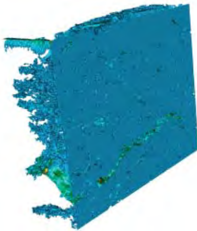
Figure 7. Steady-state flow through fractured shale based on Navier–Stokes equation. The surface plot shows the interface between pores and solid (shale). The surface is colored according to velocity magnitude in the pore, with blue representing lower velocities, shades of green, yellow, and red representing higher velocities. Resolution 48.4 nm with 1920 \times 1600 \times 640 total grid cells. Original pore structure obtained from FIB-SEM mapping, which indicates a bulk porosity of 18%. [Reproduced from Trebotich D, Graves DT (2015) An adaptive finite volume method for the incompressible Navier–Stokes equations in complex geometries Communications in Applied Mathematics and Computational Science , Vol. 10(1), p. 43–82, Fig. 13, with permission from Mathematical Sciences Publishers.]
