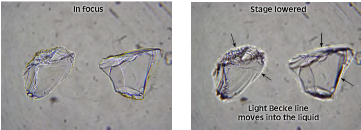
B. The grain is immersed in a liquid with n = 1.55 ; when the stage is lowered, the Becke line moves into the liquid. High relief.
