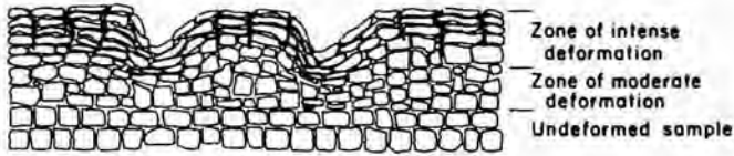
FIGURE 2.3 Schematic cross section of a polycrystalline sample illustrating the nature of deformation from the cut or coarsely ground surface down to the undeformed sample. The nature and depth of deformation varies with the nature of the sample.
