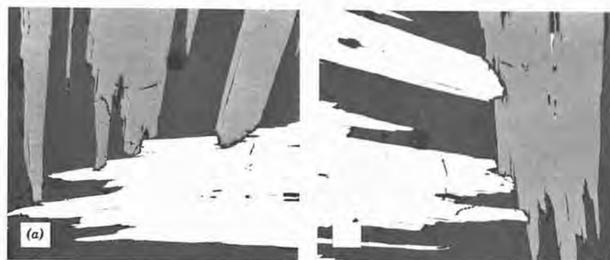
FIGURE 3.1 The properties of bireflectance and reflection pleochroism illustrated by the mineral covellite photographed in two orientations at 90^\circ to one another in plane (linearly) polarized light. The darker gray blades in the black-and-white photographs are actually deep blue; the light blades are pale bluish white (width of field = 400\ \mu\text{m} ).
