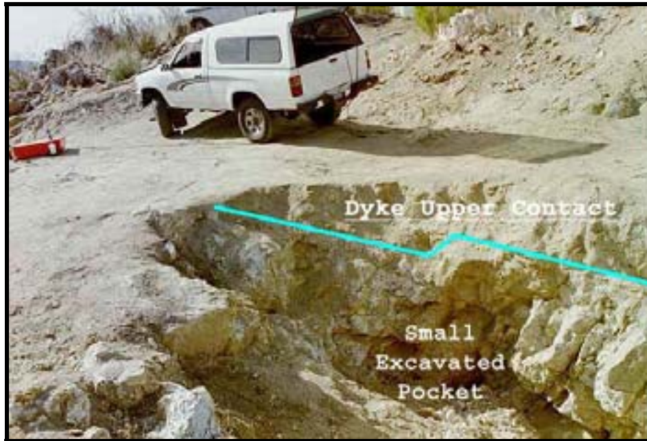
Figure 6: Outcrop of the pegmatite, northeast of the current underground workings. Dyke 1 is west dipping and approximately 1 meter in thickness at this point. The 300 MHz antenna is to the left front of the truck.
