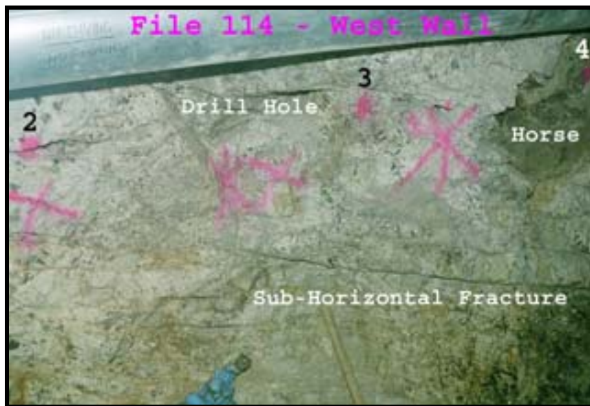
Figure 38: The West wall of the main drift, File 114. Anomaly markers are based on a real-time interpretation of the raw data at the time of the scan. Note that there are no clear geologic indicators for potential pocket mineralization along the line of scan. At the 4 th of July Pocket zone and at File 104, Lepidolite was evident in the central portion of the pegmatite. This is considered a good geologic indicator at this mine for pockets.
