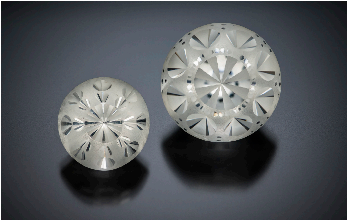
Figure 2: Compared to calcite’s birefringence of 0.124, that of quartz is relatively low at 0.009. Nevertheless, doubling will still be visible if the specimen is large enough and is viewed at the correct angle to maximize the effect. Here the larger 71.49 carat stone’s table facet is inclined approximately 45 degrees to the optic axis, there is maximum doubling, but mid-range partial birefringence. The effect is noticeable on the pavilion facets at the back of the stone as seen through its table; maximum depth is 20.15 mm at the culet (center point). The table facet of the smaller 29.39 carat quartz is cut in a plane parallel to its optic axis. Looking in a plane perpendicular to the table surface, there is maximum birefringence, but zero doubling of the pavilion facets. Both stones were cut by Art Grant and were part of the collection of Harold Dibble. The smaller stone was cut from a left-handed crystal and the larger stone is from a right-handed crystal (for more on handedness, see Skälwold and Bassett 2015); 19.20 x 15.55 and 25.50 x 20.15 respectively. Photo: Jeff Scovil.
