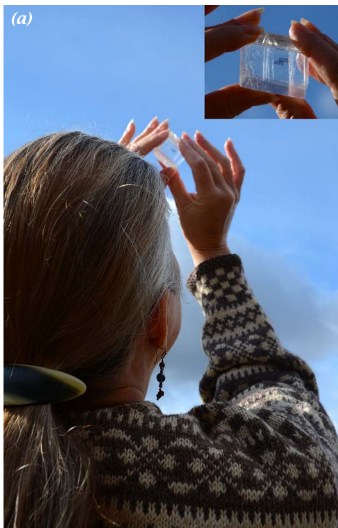
Figure 10a: The author (EAS) with a calcite cleavage rhomb and following the experiments of Leif Karlsen outlined in his book Secrets of the Viking Navigators (the rhomb is polished, but its angles are correct). Leif’s drawing in 10b illustrates the observation he used to detect the location of the sun when it is very low on the horizon and obscured by fog as is often the case in the cold waters of the arctic and subarctic ocean. The view presented is that of above the calcite, but it is “read” from below as in 10a ; in either case, the key observation is that of the equal intensities of doubled images (center). Leif devised an ingenious stand for using the sunstone; one which his Viking ancestors probably didn’t think of. Because the stone had to be “read” from below and, at the same time held level, he built a rotatable stand which employs a mirror so that the viewer need only hold it out in front and look down into the image reflected below the stone (Karlsen 2003, p.80; drawing reproduced with permission of Starpath Publications, www.starpath.com) Photo by James H. Edwards.
