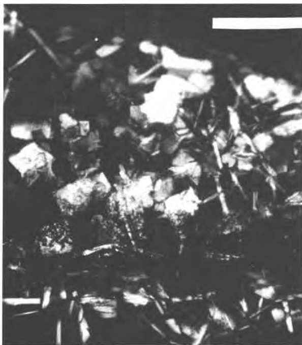
Fig. 3. Spruce Pine pegmatite plus 4.5 wt% H 2 O held at 750°C for 96 h. The capsule wall was in the upper left corner. Scale bar = 1.0 mm; cross-polarized light.
