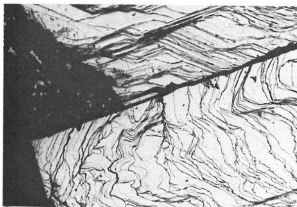
FIG. 3. General view of crystal face exhibiting two blocks outlined by surfaces closely parallel to the cubic faces (100). The growth steps in the two blocks are of different types. On the upper block the steps are straight and regular and are parallel to the (100) and (320) faces. On the lower block the steps are of warped and irregular outline but tend to develop into (100) and (320) faces. The blocks are separated by a split in the crystal faces. \times 75 .
