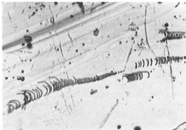
FIG. 6. Linear series of dislocations lying nearly parallel to the (320) faces. \times 750 .
