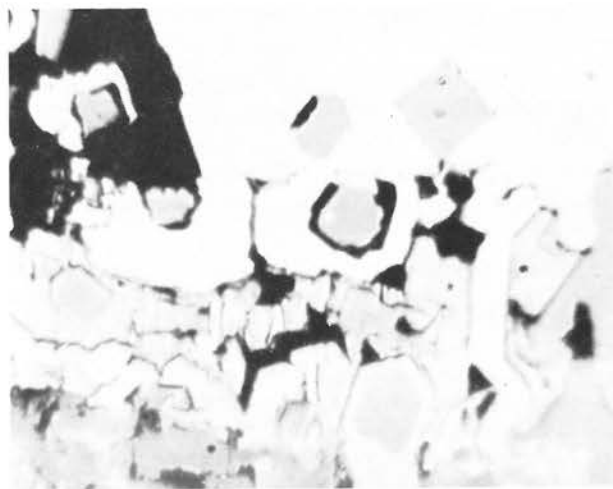
FIG. 2. Bravoite grains (dark gray) enclosed in siegenite (upper right, medium light gray), and in galena (gray). Type I zoning. Oil immersion, 550X.
