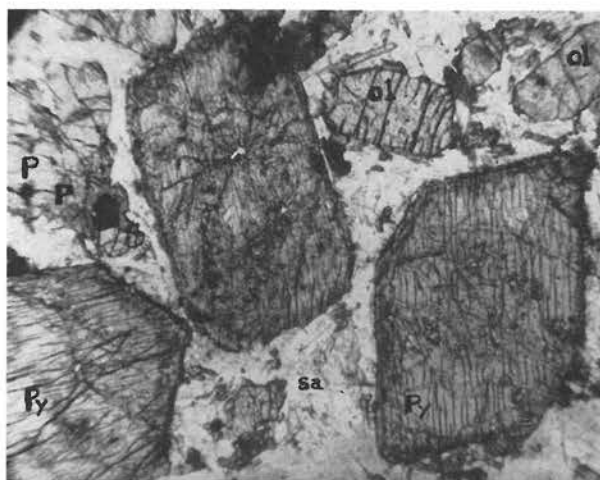
FIG. 4. Interstitial massive sanidine, Sa=Sanidine, Py=Pyroxene with reaction rims, Ol=Olivine, P=Phlogopite. Nicols not crossed, \times 26 .
