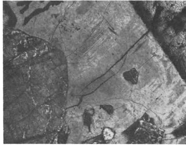
FIG. 8. Interstitial massive sanidine with brown pleochroic patches and faint lamellae. Nicols crossed, \times 70
