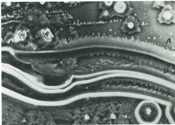
FIG. 8. Photomicrograph showing the existence of stacking fault in silicon carbide crystal. Positive phase contrast, \times 1000 .
