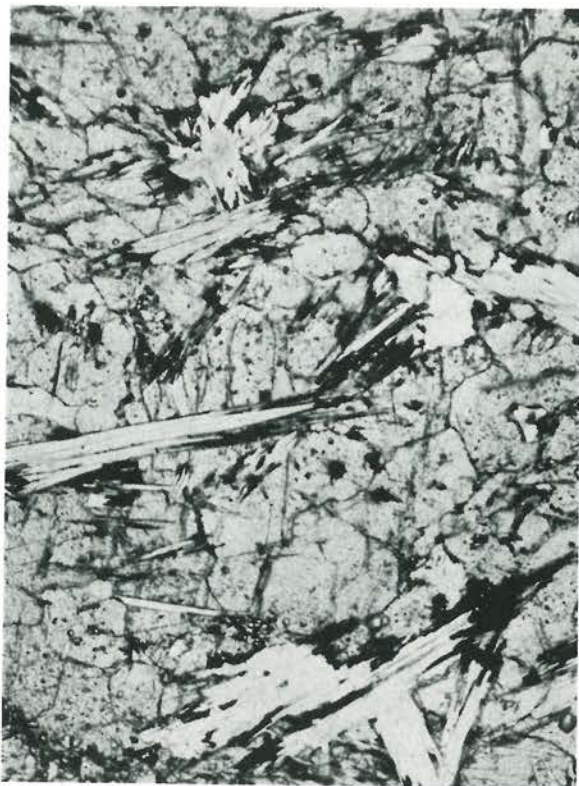
FIG. 16. Nearly monomineralic fayalite being replaced by prismatic cummingtonite. Secondary magnetite (black) is developed at the margins of some of the cummingtonite grains. (Plane light, \times 31 )
