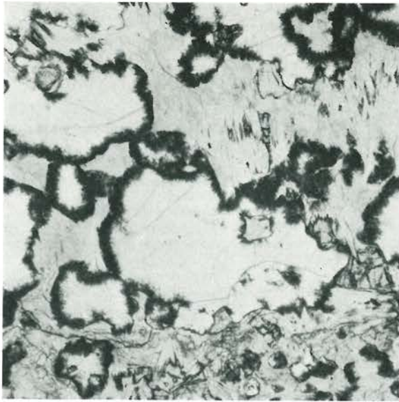
FIG. 18. Masses of fine-grained prismatic and fibrous cummingtonite (grey, moderate relief) and surrounding rims of acicular cummingtonite (dark-colored) developed in a quartz-rich layer at its boundary with a layer of ferrohypsthene-fayalite taconite. (Plane light, \times 32 )
