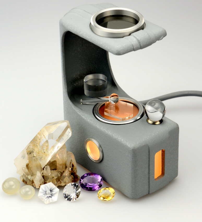
Figure 3: There are various ways of viewing specimens between polarizing filters. One is to use a polariscope, such the model at left. A fixed filter termed the polarizer is at the bottom and a rotatable filter termed the analyzer is at the top. Transmitted light is provided by a bulb in the base (or by an external light for other models). A similar setup may be used in microscopes either with provided filters or by using a portable polariscope resting on the stage. The sphere on the end of the glass rod is strain-free and is used to resolve the optic figure; a 10x loupe works just as well. A number of test specimens are shown, including 3 mm and 14.75 mm basal sections and a 10 mm sphere (all on the stage); faceted purple, yellow and colorless quartz specimens – the latter two optical-quality quartz were optically oriented by the author (EAS) and custom cut by Mark Oros. The two milky white cabochons from Sri Lanka feature multi-star networks; using the bull’s eye to orient them makes it easy to study their fascinating intricate networks, especially in spherical versions.
