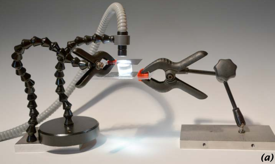
Figure 6a: A simple setup for observation of optical activity in quartz; essentially an upside down polariscope. Polarizing filters may be purchased from a supply catalog or removed from a pair of old sunglasses. Figure 6b: Thickness affects the colors seen in the center. In contrast to Fig. 1, a 14.75 mm thick basal slice produces a red > yellow > green bull's eye color sequence when the filter is turned clockwise, indicating that it is likely an optically right-handed crystal; confirmed with observation using a quarter-wave plate or a very thin cleavage wafer of muscovite mica.
