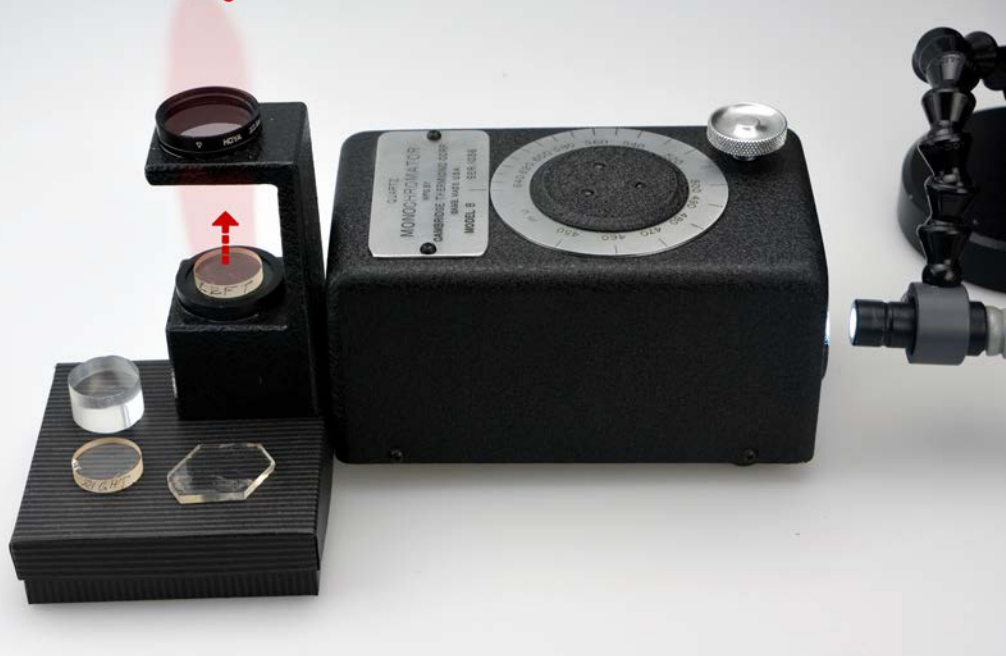
Figure 10: The narrow bandwidth of light generated by the quartz monochromator is useful in a number of applications. With the dial set to 650 nm, it is shown here selecting red light from the white light generated by the fiberoptic source at far right. A portable polariscope with its rear light port lined up with the exit port of the monochromator directs the beam up through the polarizer, a 4 mm left-handed basal section of quartz and the upper filter to the viewer. By rotating the upper polar (analyzer) of the polariscope one can make refined observations of the optical activity in quartz specimens, including illustrating the values of Table 1 by noting how many degrees the analyzer must be turned for each wavelength of color listed. Pictured are the 3 mm and 14.75 mm thick basal sections shown earlier, along with two 4 mm thick basal slices, one each of left and right-handed quartz.
