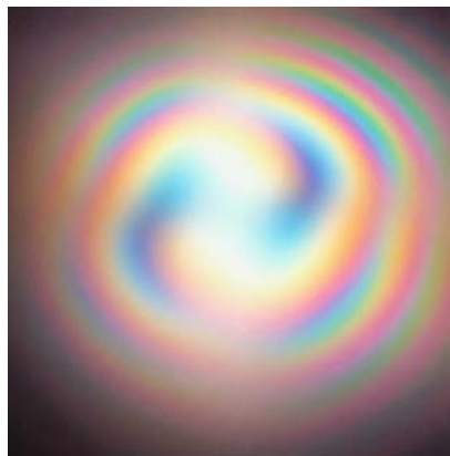
Figure 5: Above: a quarter-wave plate with right or left-handed spiral as seen through its round window when placed between crystal and analyzer. Below: Airy's spiral in the 3 mm left-handed basal section of figure 1.
