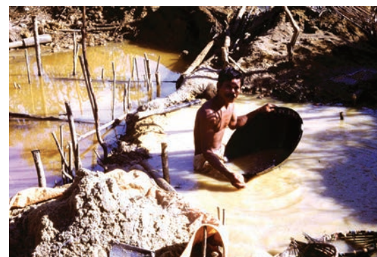
Figure 63. Younger Holocene gravels being concentrated using wooden cone-shaped “pans”, around Cempaka, Indonesia.
