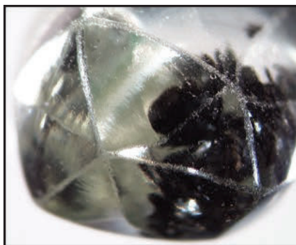
Figure 43. An alluvial diamond from the Urals (Russia) showing abrasion of the edges of a tetrahedron with lesser damage along the medial lines. [Image by Jeff Harris.]
