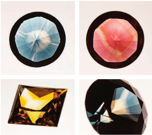
Figure 31. Distinctive color zoning in faceted HPHT diamonds stemming from growth sector dependent impurity distributions. [Used by permission of the Gemological Institute of America, from Shigley et al. (2004b) Gems and Gemology , Vol. 40, Fig. 5, p. 307.]
