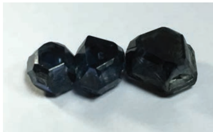
Figure 13. Deep blue to black Type IIb HPHT diamonds grown on {111}-oriented diamond seeds. Sizes range from approximately 6 to 15 ct. The upper face has a {111} orientation, reflecting that of the seed. The sizes and orientations of the other faces depend on the pressure and temperature conditions in the growth cell. [HPHT diamonds synthesized and photographed by ANK.]
