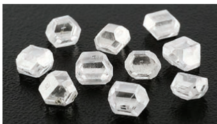
Figure 6. HPHT diamond crystals (0.5–0.69 ct) grown by Jinan Zhongwu New Materials Company Ltd. of Shandong, China, showing characteristic cuboctahedral growth morphology. [Used by permission of the Gemological Institute of America, from Eaton-Magaña et al. (2017) Gems and Gemology , Vol. 53, Fig. 2, p. 266.]
