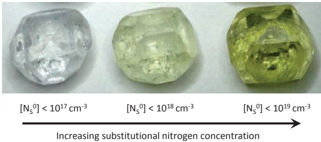
Figure 12. Nitrogen doping influences the color of HPHT diamonds, with yellow color being observed with increasing isolated substitutional nitrogen concentrations ( [N_S^0] ). These concentrations were controlled by including nitrogen getters in the growth capsule. Each diamond crystal is ~7 ct in size. [HPHT diamonds synthesized and photographed by ANK.]
