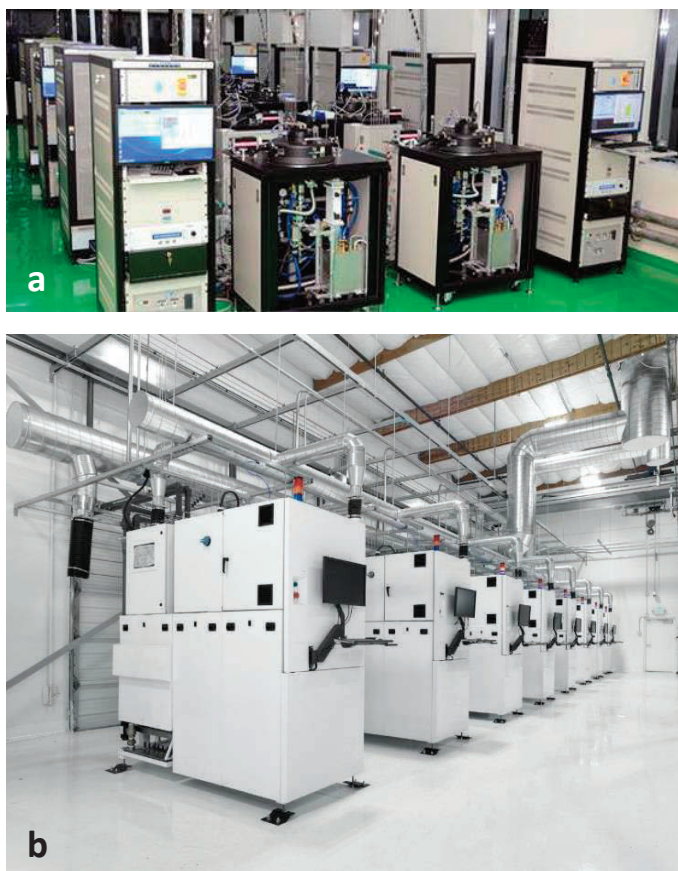
Figure 26. (a) A CVD diamond growth facility based on commercially available tools; and (b) A CVD diamond growth facility based on proprietary designed tools. [Used by permission of (a) ABD Diamonds Pvt. Ltd. and (b) Diamond Foundry, Inc.]
