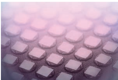
Figure 25. Multiple single crystal seeds growing in a CVD diamond reactor. [Used by permission of Element Six (UK), Ltd. and Lightbox Jewelry, Inc.]
