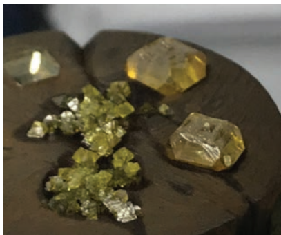
Figure 9. The simultaneous presence of optimal and over-saturated carbon flow during the HPHT diamond growth process resulted in the formation of high quality flat-surfaced single crystals ( upper right ) and multi-crystal aggregates (druzes, lower left ) due to growth instability, respectively. The larger crystals weigh approximately 4 ct. The diamond materials are here imbedded in the remains of the growth medium after a short acid clean. [Diamonds grown by ANK with Alkor-D Ltd. Photograph by ANK.]
