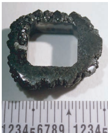
Figure 23. The polycrystalline rim of a CVD-grown single crystal after laser coring. [Photograph by JEB.]
