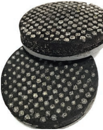
Figure 11. Typical example of HPHT diamonds resulting from multiple seed and multiple layer growth methods. The view is from the seed side (the bottom of the reaction volume illustrated in Fig. 2b), where the growth medium has been partially dissolved by acid cleaning. Average crystal size is ~4 mm each. [Diamonds grown and photographed by ANK.]
