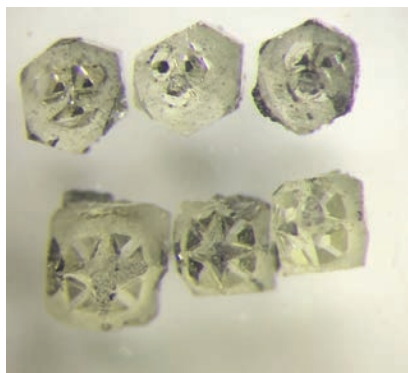
Figure 14. Example of extremely rare HPHT diamond single crystals with pure rhombic dodecahedral {110} external morphologies. The upper and lower rows show crystals with 3-point and 4-point joining tips, respectively. The light yellow hue of the crystals is a result of nitrogen doping occurring due to loss of nitrogen-getter efficiency at high growth temperatures (>1850 °C). [HPHT diamonds grown by ANK with Alkor-D Ltd. Photograph by ANK.]
