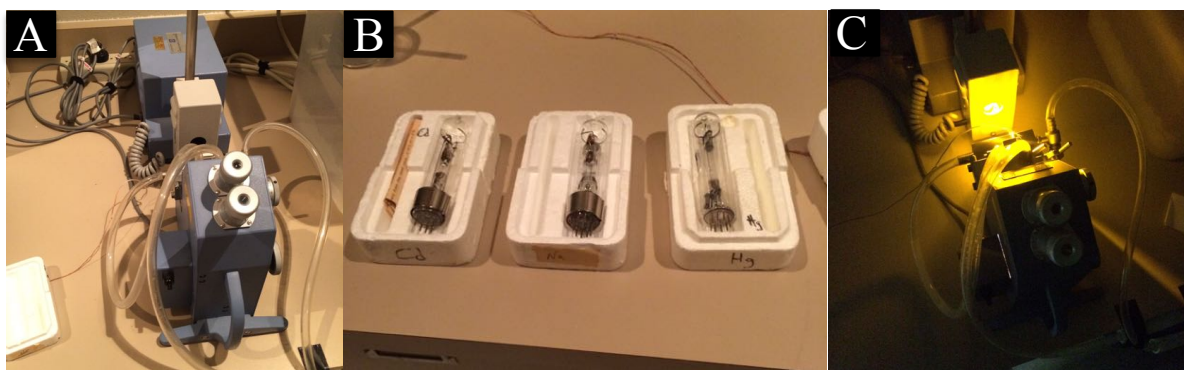
Figure 6.3 (A-C) (A) Refractometer, (B) gas discharge bulbs, (C) and light source of the refractometer.
