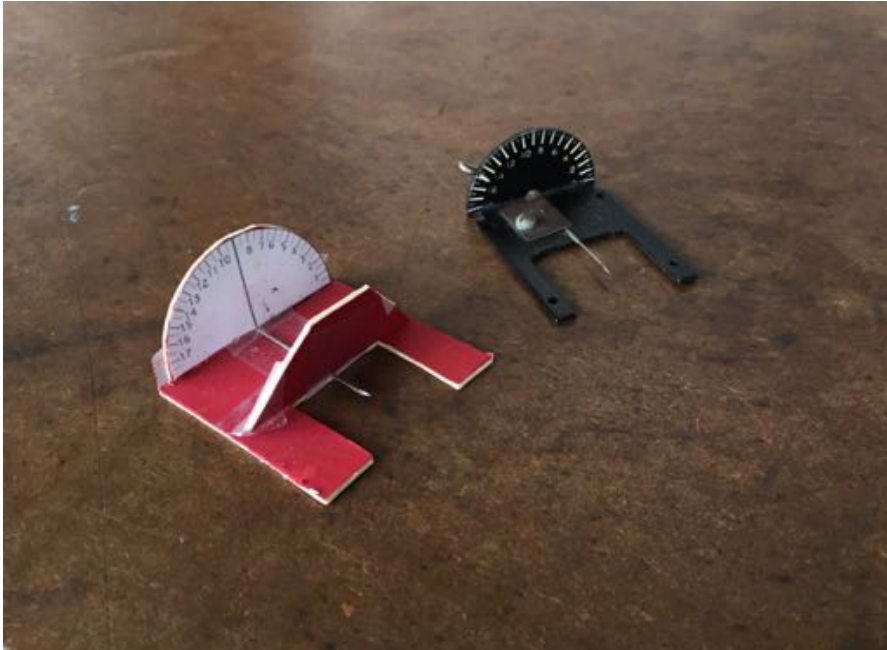
Figure 2.4 Homemade (left) and detent or “Wilcox”(right) spindle stage. Research quality orientation solution may be collected using these stages as well (Gunter, 2004).
