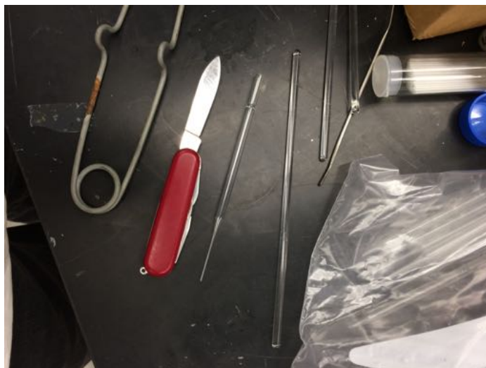
Figure 3.2 Cutting tool and glass starting material for pulling fibers.
