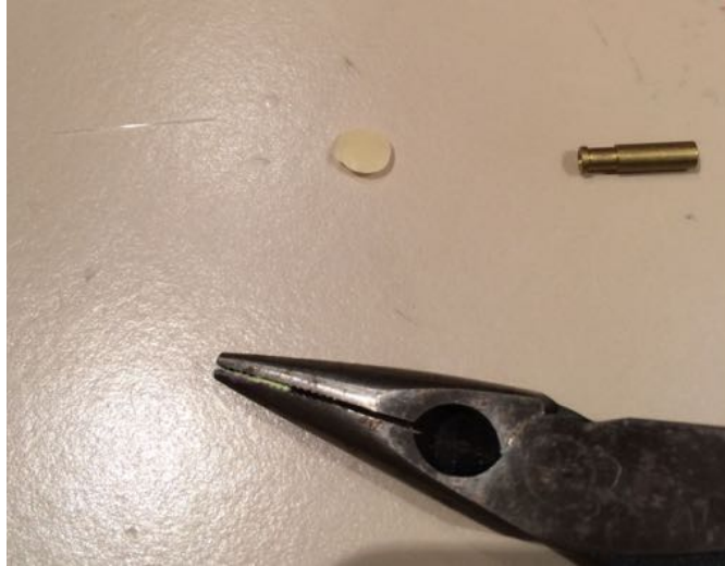
Figure 3.9 Glass fiber, beeswax, and Supper specimen pin fit for optical and/or x-ray goniometers.
