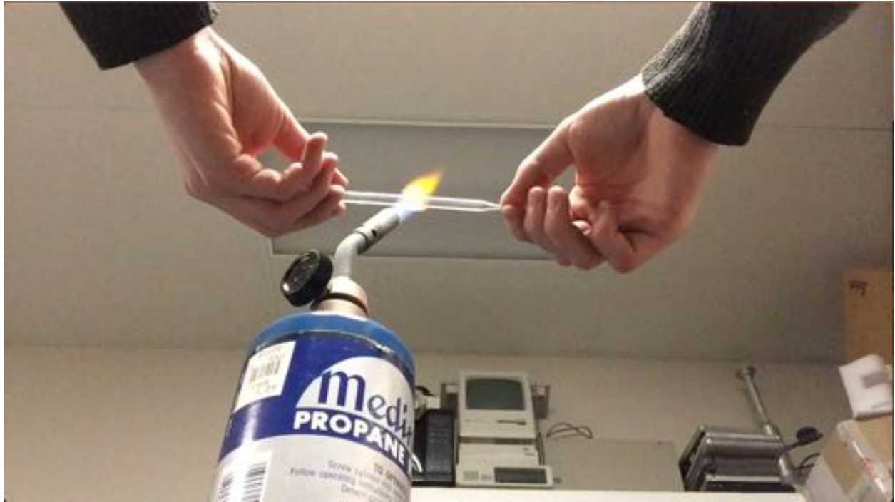
Figure 3.3 Under the torch, the glass starting material will burn orange and a glass dropper tube like this takes about 30 seconds to become pliable.
