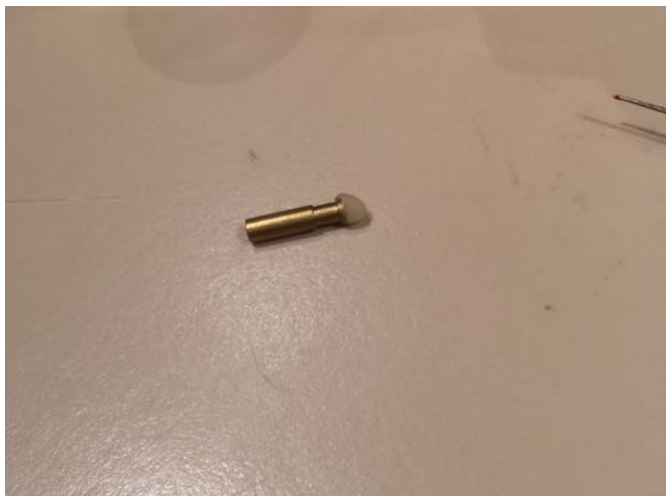
Figure 3.10 Specimen pin with beeswax. Plasticine may also be used in place of beeswax.
