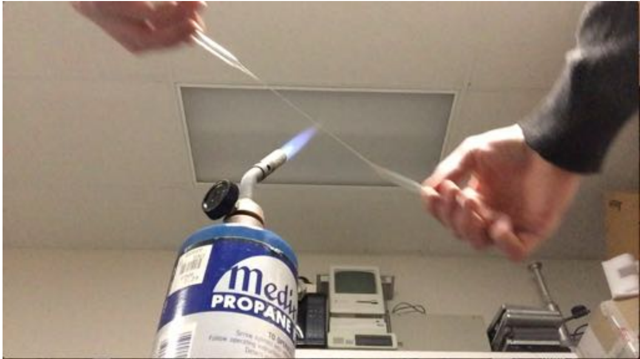
Figure 3.5 Pulling the fiber too slow will result in thick fibers and pulling too fast results in pulling the glass apart. The key is to have the right pliability and constant speed of pull.
