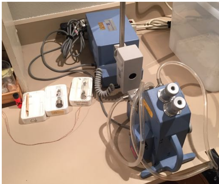
Figure 2.6 Bellingham and Stanley Abbe 60 refractometer. This is a high precision refractometer that can be used for refractive index liquid calibration. The word ‘calibration’ is used in this context to describe accurately measuring refractive index of a Cargille liquid at multiple wavelengths to model its dispersion.
