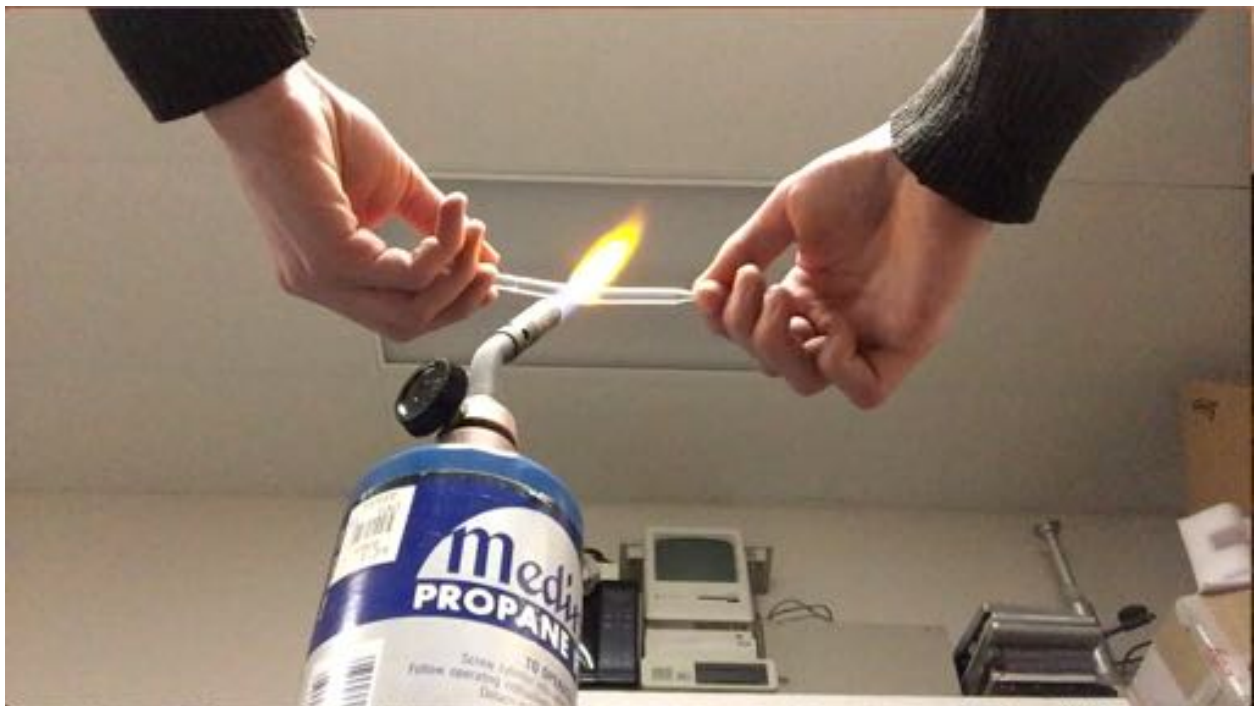
Figure 3.4 Somewhere between the point where the glass becomes pliable, and the point where it is totally molten is when the glass is ready to be pulled. Finding this point takes practice but there should be some resistance in the glass, otherwise it will fall apart.
