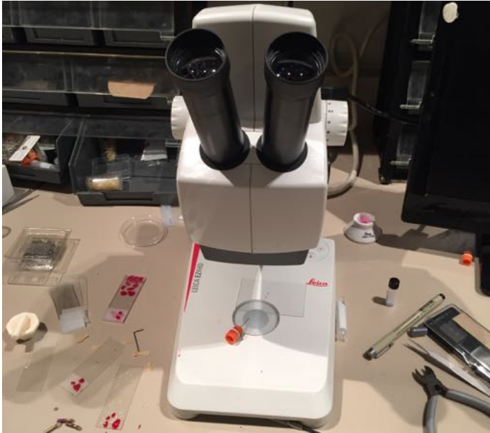
Figure 2.2 Leica stereoscope used for mounting crystals. Crystals are sorted on glass slides and adhered to a specimen pin with nail polish.
