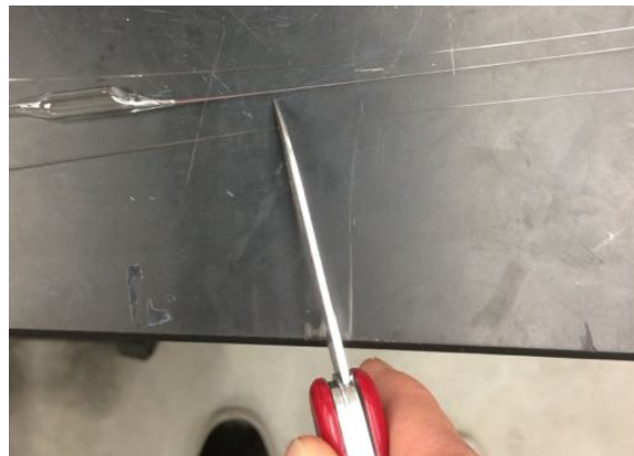
Figure 3.6 With long thin strands of glass, fibers can be sectioned with a cutting tool
