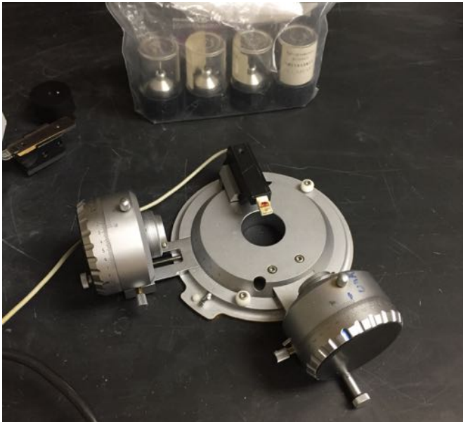
Figure 2.3 Micro-refractometer spindle stage made by Olaf Medenbach. When used with a dispersion-staining lens, this spindle stage can be used to plot dispersion curves without the use of a monochromator.
