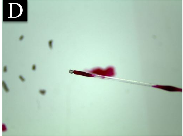
Figure 3.18 A-D (A) Placing nail polish behind the crystal, (B) pulling back on the fiber to immerse the tip in nail polish, (C) driving the fiber through the nail polish and into the crystal, and (D) pulling the fiber and crystal straight up off of the slide.
