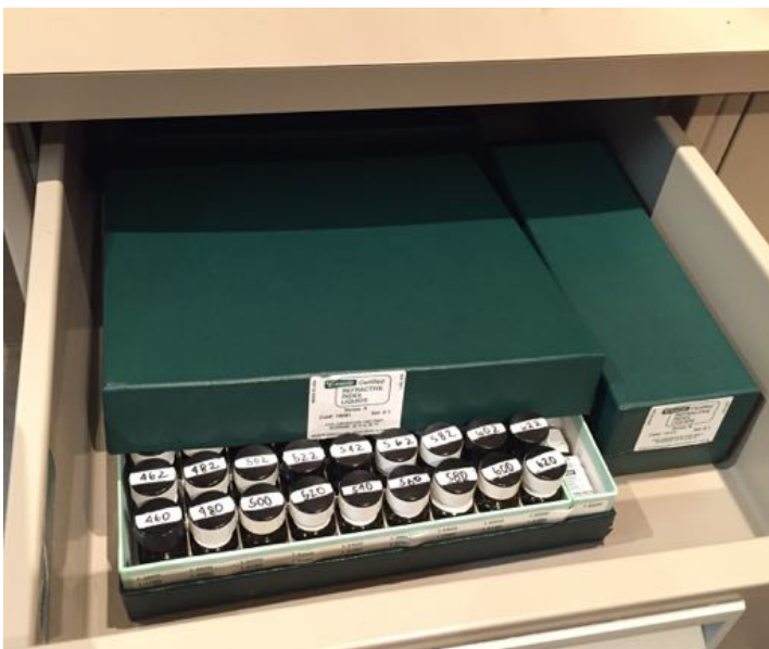
Figure 2.5 Boxes of Cargille refractive index liquids. With relatively new refractive index liquids, the values on the label are very accurate and can be used without calibration. These are essential to measuring refractive indices of minerals, and are helpful for seeing extinction positions in XPL.
