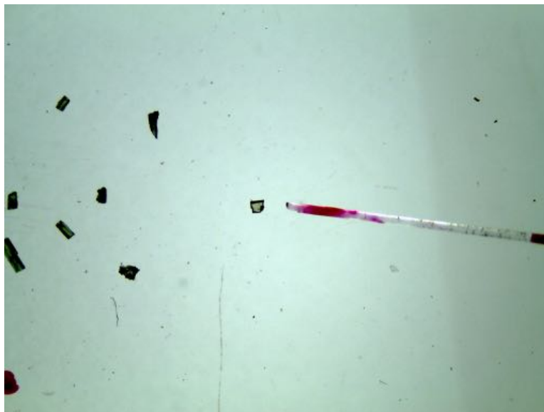
Figure 3.16 Comparison of the glass fiber diameter to the diameter of the crystal of interest.
